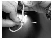
3 - Slowly pull the end tip of the seal to the desired aperture.
