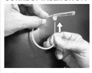
1 - To close the seal, hold the end tip of the thread and push it through the locking mechanism.
