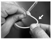
4 - Make sure you hold the seal on its very end while inserting. Holding the seal on the middle of the thread may cause weaknesses to it.
