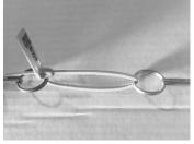
6 - The pullock seals are meant to indicate tampering and not to hold the compartment closed. When the seal is used on its last locking point under stress, as per picture below, the seal may accidentally break.
